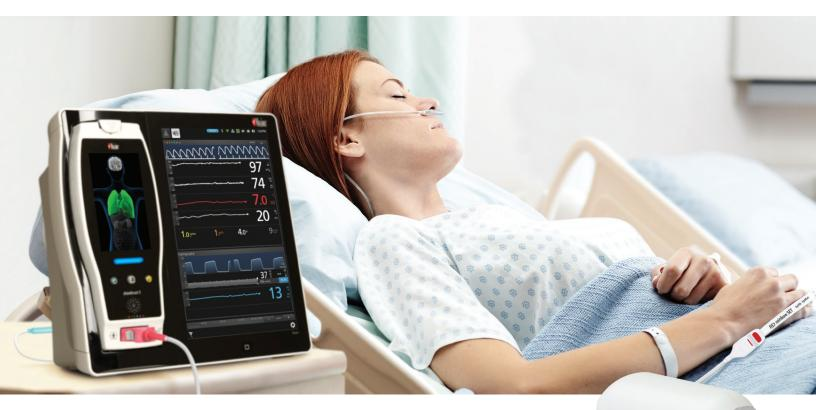
NomoLine infrared sidestream gas analyzers provide end-tidal carbon dioxide and multigas measurements (oxygen, nitrous oxide, and anesthetic gases) in a variety of clinical settings for all patient populations
